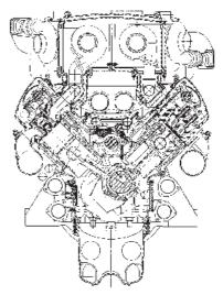
engine block. The liner is trapped between the crankcase and the cylinder head at the liner flange. The lower support for the liner is arranged to be high in the crankcase and incorporates two 'O' ring seals and a large 'wedge' ring.
